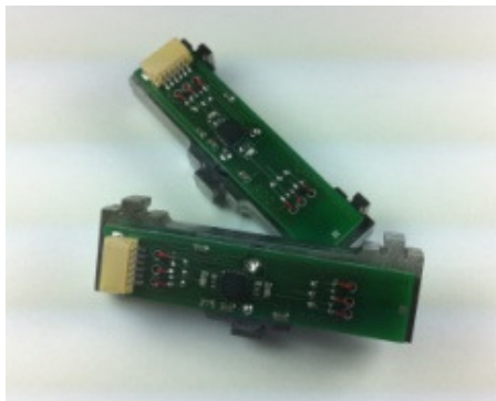
Figure 6: Mini double Shear-beam sensors arranged in a 80 measurement point matrix
