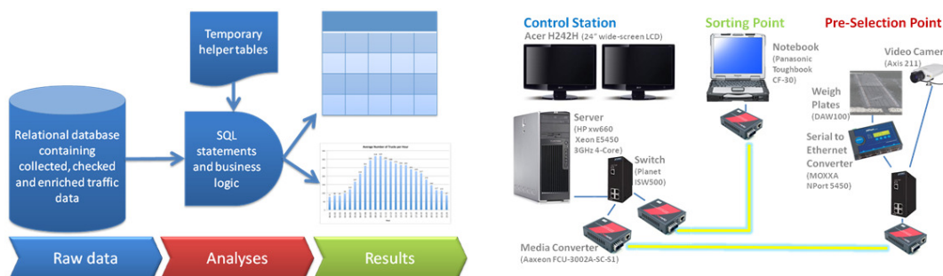
Figure 22: Hardware/software framework for capturing real-time traffic data for German test site
